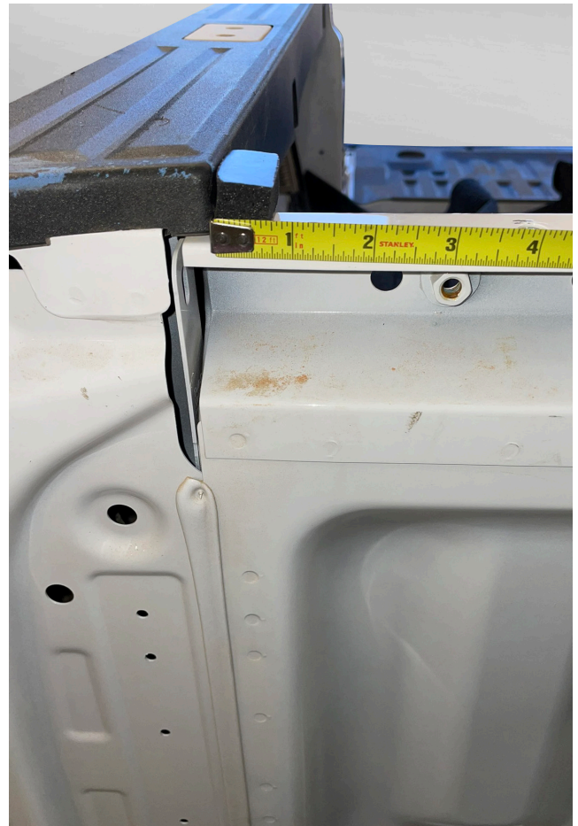
10. Cut 1" piece of foam seal tape and place on bulkhead against cap rail. Repeat on other side
