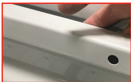
Clean top surfaces of bed and bed caps.
