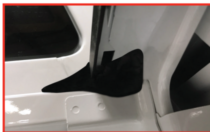
Compact putty/butyl tape and create a transition from bed cap to front rail.
