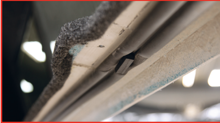
Spacer position, shown close-up, should be removed.
