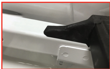
Compact putty/butyl tape and create a transition from bed cap to front rail.
