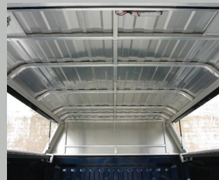
TIG welded Super Cage roof construction
