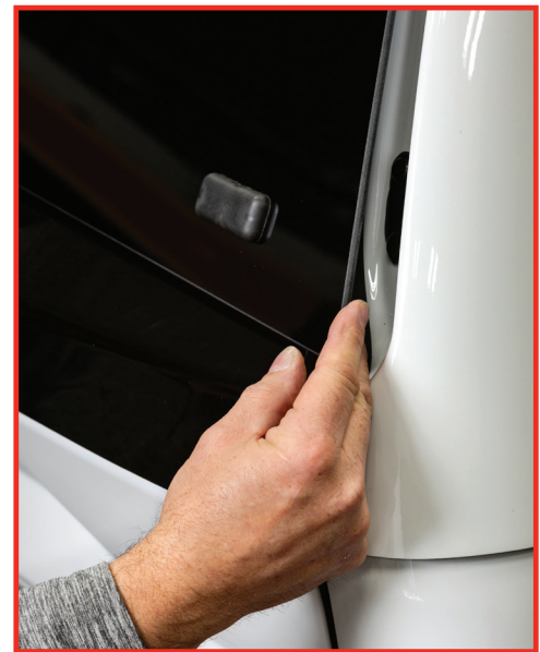
Fig B. Check fit & function of door, handle & seals.
