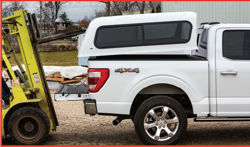
Open truck tailgate and rear door of cap, using a forklift or (4) people place the cap on the truck.
