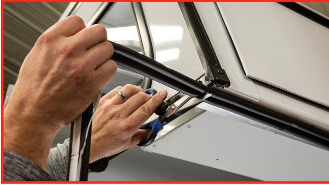
Fig. A Starting at the driver side rear, apply the double bulb seal 5/8" from the outside cap edge in a straight line toward the front.
