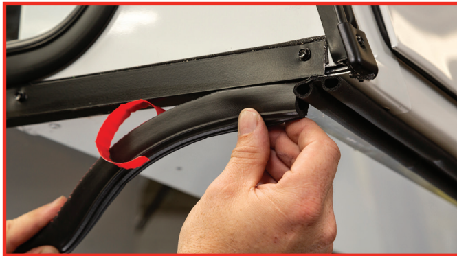
Fig. B. Apply the bulkhead seal to the front underside of the cap, butting up to both the driver and passenger side double bulb seal.
