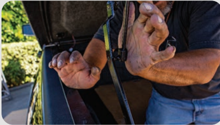
[10] The hinges are secured to the brackets on the side bed rails, and the gas struts are secured from the lid to the brackets.
