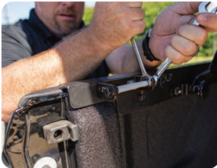
[10] The hinges are secured to the brackets on the side bed rails, and the gas struts are secured from the lid to the brackets.
