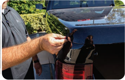
[09] The SnugLid SL is placed over the bed and adjusted until an even one-finger gap all around is achieved.
