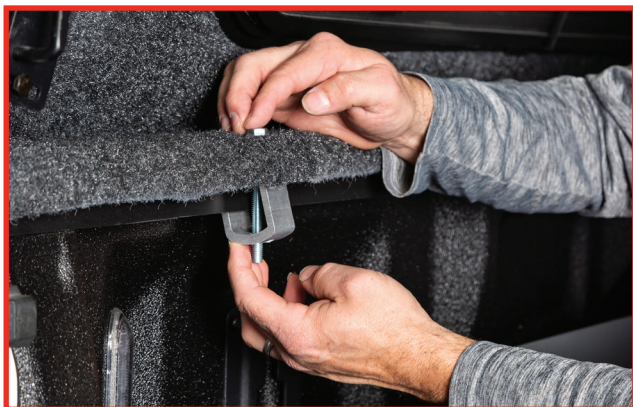
Place clamp bolt with washer through J-Bolt pockets in cap. Align J-Clamp as shown. Insert washer and nut, then tighten bolt. Repeat at all (4) locations.
