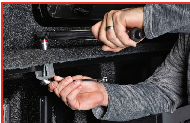
Tighten clamps to specified torque.
